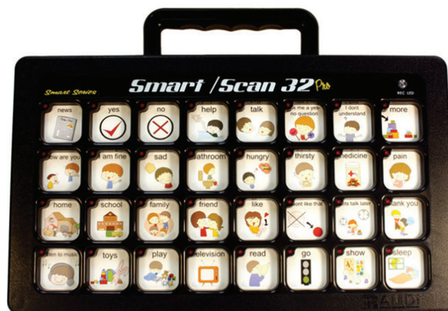
Fig. 1: Smart/Scan 32 pro, an augmentative communication device
