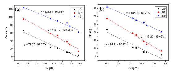
**Figure 7.** Gloss as a function of surface roughness (**a**)  $S_a$  and (**b**)  $S_q$  calculated from 5000  $\mu$ m × 5000  $\mu$ m images.
