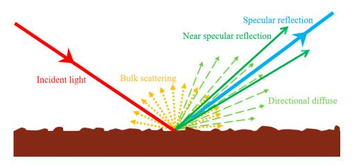
Figure 1. A systematic illustration of light scattering at a randomly micro rough surface.
