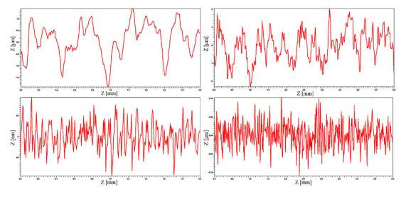
**Figure 4.** Surface profile curves of typical *PU2* and *PU4* films extracted from the above Figure 3. Upper images are corresponding to *PU2* and lower images to *PU4* film.
