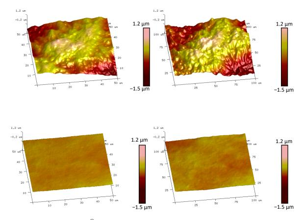
**Figure 5.** AFM ScanAsyst<sup>®</sup> mode height images of *PU2* and *PU4* at 50  $\mu$ m × 50  $\mu$ m and 100  $\mu$ m × 100  $\mu$ m measurement lengths, respectively. Upper images are corresponding to *PU2* and lower images to *PU4* film.
