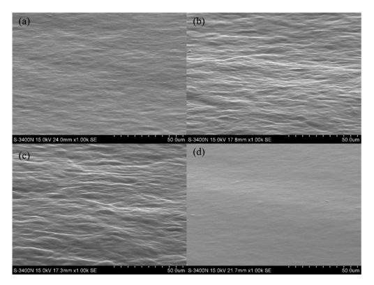
**Figure 2.** SEM topographic images of *PU1*, *PU2*, *PU3*, and *PU4* films, respectively. The CO contents are (a) 1.72%, (b) 3.44%, (c) 5.16%, and (d) 6.88%, without the addition of phenolic epoxy resin.
