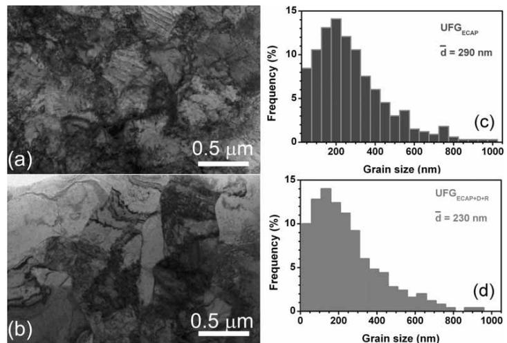
**Figure 2.** a,b) Typical bright-field TEM images for the  $UFG_{ECAP}$  and  $UFG_{ECAP+D+R}$  Cu samples, respectively. It is apparent that the grain boundaries in the  $UFG_{ECAP+D+R}$  sample are sharper and straighter than in the  $UFG_{ECAP}$  sample. c,d) Grain size distributions measured from TEM images for the  $UFG_{ECAP}$  and the  $UFG_{ECAP+D+R}$  samples, where  $\bar{d}$  is the average grain size.
