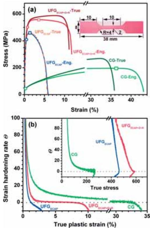
**Figure 1.** a) Tensile engineering and true stress–strain curves of the  $UFG_{ECAP+D+R}$ ,  $UFG_{ECAP}$ , and coarse-grained (CG) Cu samples.  $\square$ : uniform elongations,  $\circ$ : 0.2% offset yield strengths. Inset: dimensions of the tensile sample with a thickness of 0.1 mm.  $R$  is the radius of the arc designated by the arrow. b) Normalized strain-hardening rate ( $\theta$ ) against true strain. Inset: curves of  $\theta$  against true stress.
