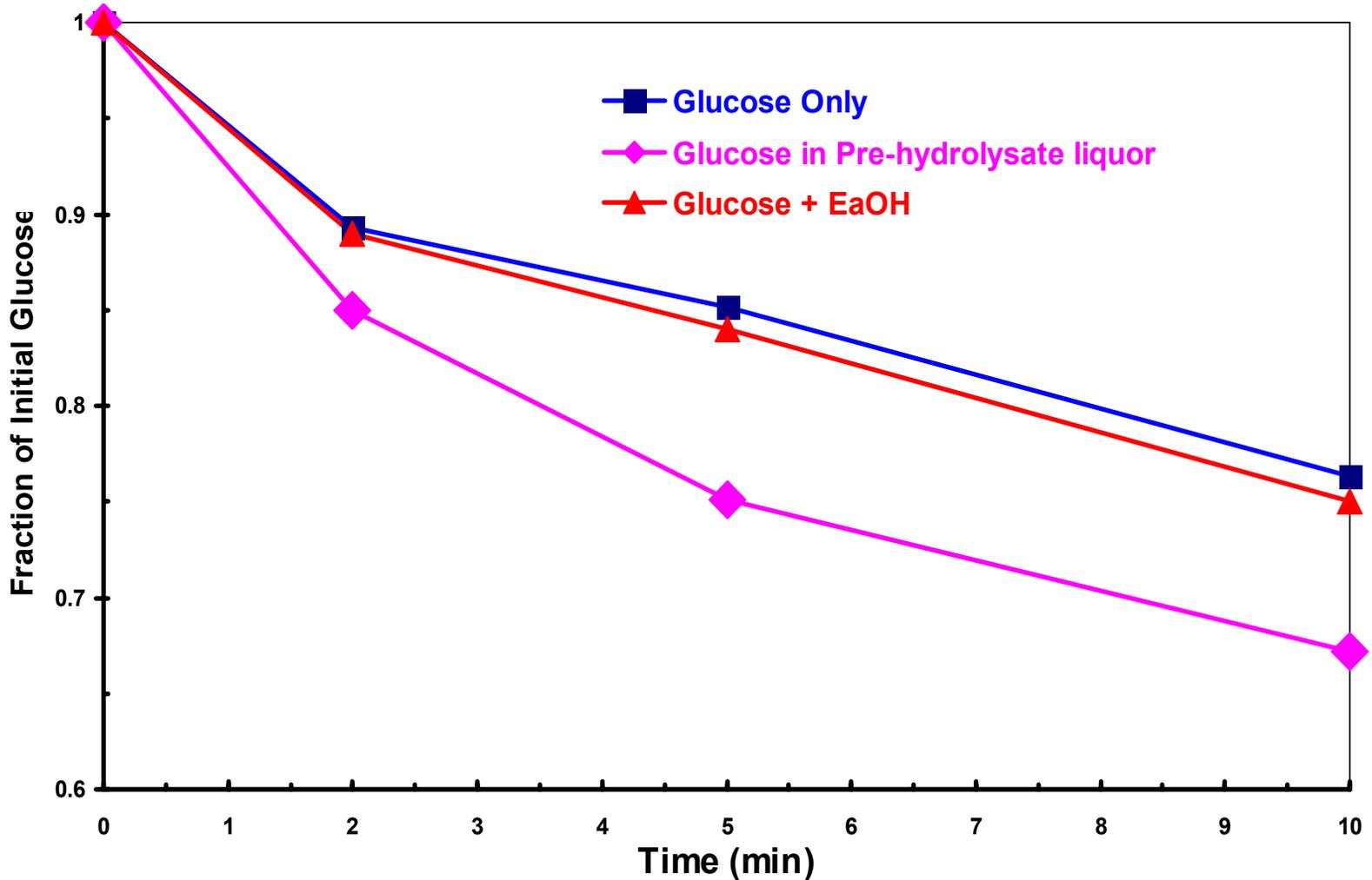
**Glucose decomposition under different medium and condition of pH=2.0 and temperature=200°C. Pre-hydrolysate liquor contains acid soluble lignin.**
