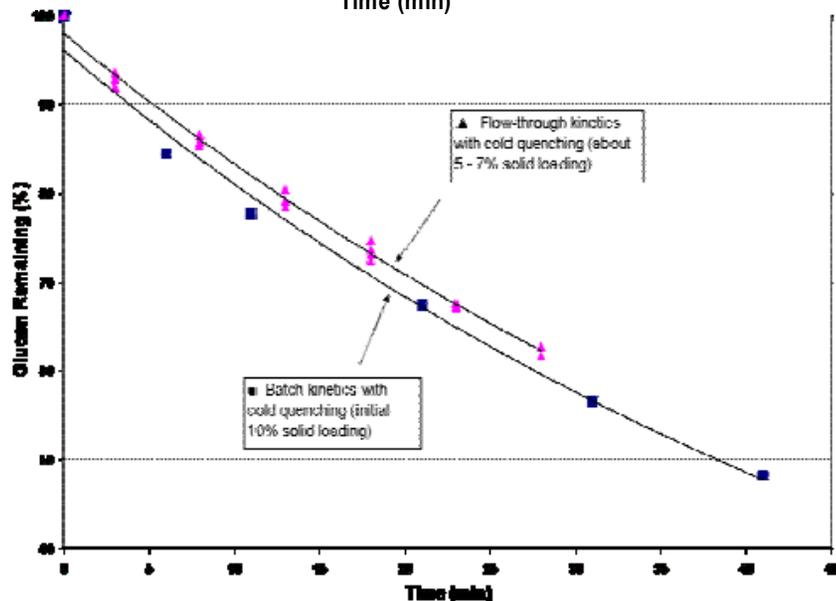
■ **Hydrolysis rates are identical for batch and flow-through reactors with no lignin but 2-3 times different when acid-soluble lignin (ASL) presence.**
