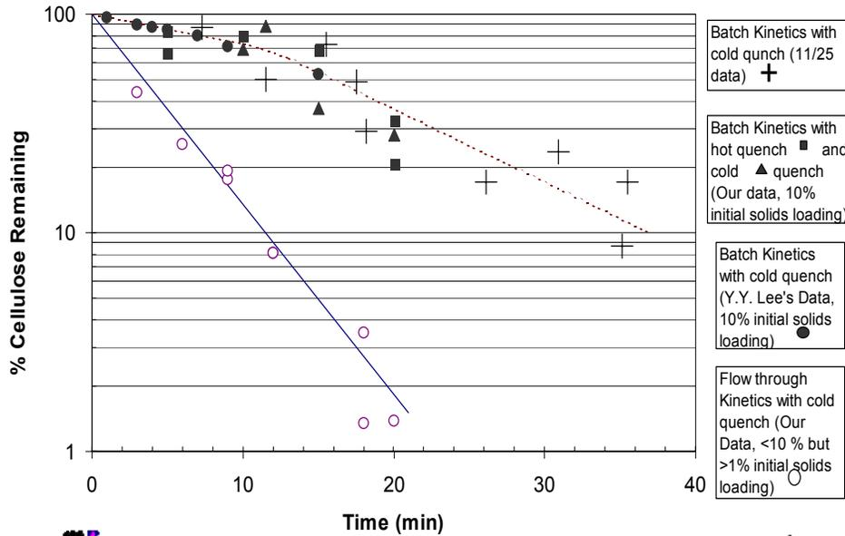
**UP: Comparison between batch and flow-through reactor (R. Torget, 1998). Pretreated yellow poplar (with lignin and xylan free) hydrolysis kinetics at 225 oC, pH 2.2.**
