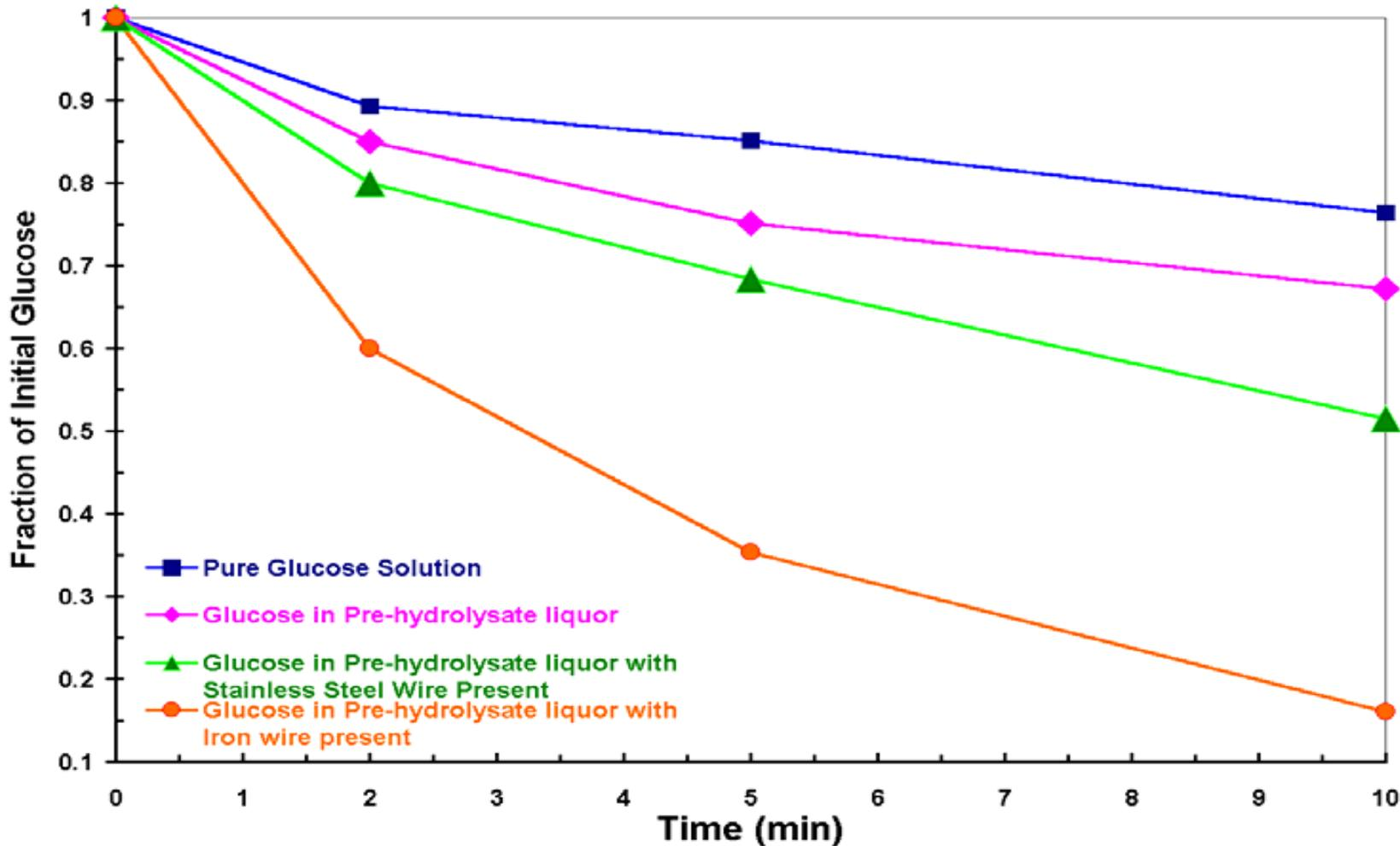
**Glucose decomposition in presence of different metals and under pH=2.0 and temperature=200°C. This study simulates the actual glucose decomposition under acid hydrolysis process**
