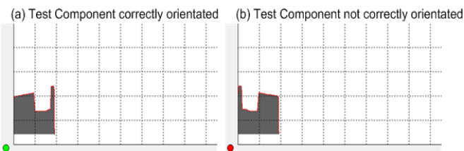
Fig. 4 Example of camera images during the optical recording of the test specimen
