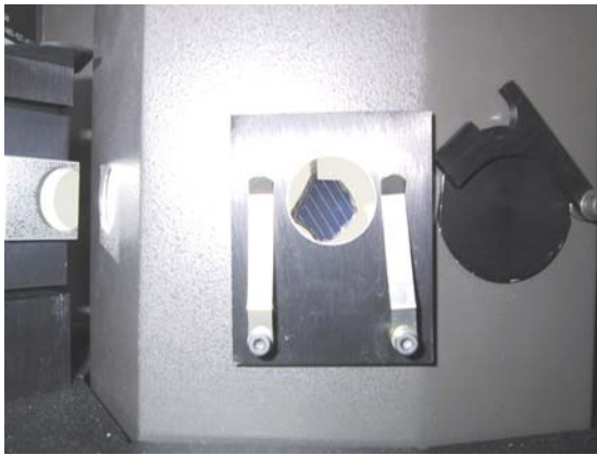
Figure 6: PV module sample during the reflectivity measurement
