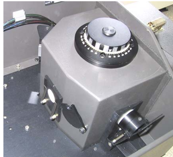
Figure 4: Labsphere RSA-PE-19 reflectance spectroscopy accessory and Spectralon integrating sphere
