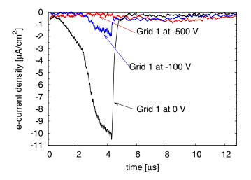
FIG. 8. (Color) Measured instantaneous electron current density into the wall of a train of 43 proton bunches, 108 ns apart, with an average bunch intensity of  $1.6 \times 10^{11}$ . With increasing voltage on grid 1, electrons below certain energies are rejected, allowing the measurement of electron energy spectrum in the cloud [43].
