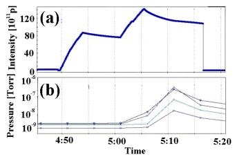
FIG. 24. (Color) Increase of gas density in cold arcs (b), as measured by 4 gauges, when protons are injected (a). The increase of the gas density is measured with a warm gauge connected to the cold vacuum through a small diameter conduit.
