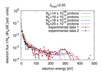
FIG. 11. (Color) Energy spectrum measured, and simulated for  $\delta_{\text{max}} = 2.05$  and different bunch intensities. The spectrum shape is not significantly affected by the  $\delta_{\text{max}}$ , but depends on the beam parameters (bunch intensity, length, etc.) [21,22].
