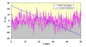
FIG. 21. (Color) Single slice of a  $0.2 \text{ mm} \times 50 \text{ mm}$  surface scan of RHIC beam pipe material obtained by Solarius, Inc. [83] using an optical profilometer. An ion trajectory incident at 1 mrad is superimposed, showing multiple transitions between vacuum and solid [25].
