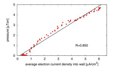
FIG. 10. (Color) Pressure increase vs time-averaged electron current density into the wall. Red dots are measured values, the black line is a linear fit [21,22].
