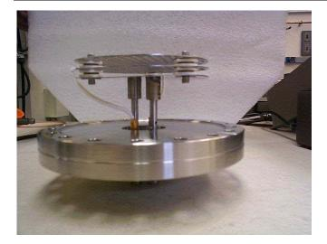
FIG. 7. (Color) Multigrid electron detector in RHIC. The grids have a diameter of 12 cm [43].
