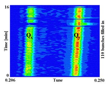
FIG. 6. (Color) Coherent tunes of the last injected bunch along a train of 110 proton bunches with 108 ns spacing in the Yellow ring. Because of coupling both transverse tunes are visible [20].
