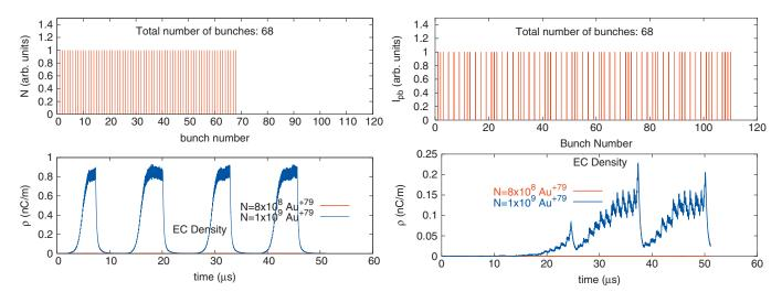
FIG. 19. (Color) Simulated electron cloud evolution over 4 turns for 68 Au bunches with a single gap of maximum lengths (top), and 68 bunches distributed approximately uniformly around the circumference [74].
