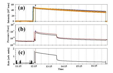
FIG. 4. (Color) Pressure rise in the PHOBOS experimental area after rebucketing with 56 bunches. The beam intensities in the Blue and Yellow ring (a) slowly decay during a store, and the pressure measured in 2 gauges (b) drops sharply after some time. With high pressure the experimental background (c) is increased [33].
