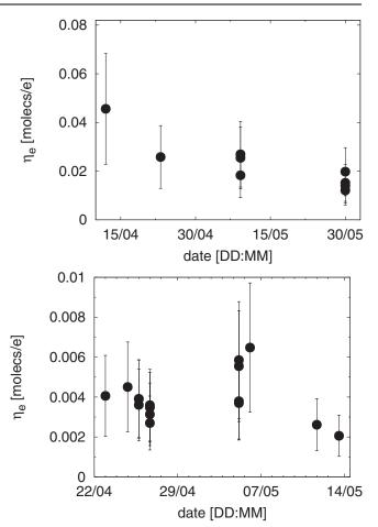
FIG. 12. Calculated desorption coefficients for the unbaked stainless steel surface BO2 (top), and the baked stainless steel surface at IR12. The error bar (50%) stems from the systematic uncertainty in the pumping speed and vacuum pressure readings. A decrease of the desorption coefficient with time is noticeable for the unbaked stainless steel (top) due to the scrubbing effect [21,22].
