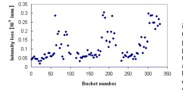
FIG. 13. (Color) Yellow beam loss at transition as a function of position in the bunch train. In this pattern 8 bunches are missing after 1/3 and 2/3 of the bunch train length. The bunch train is followed by the abort gap. The intensity losses per bunch increase until a gap is reached, and then fall back because the electron cloud decays.
