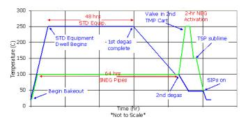
FIG. 16. (Color) Typical NEG section bakeout and activation. After all surrounding components have been baked at 250°C, the NEG surface is activated.
