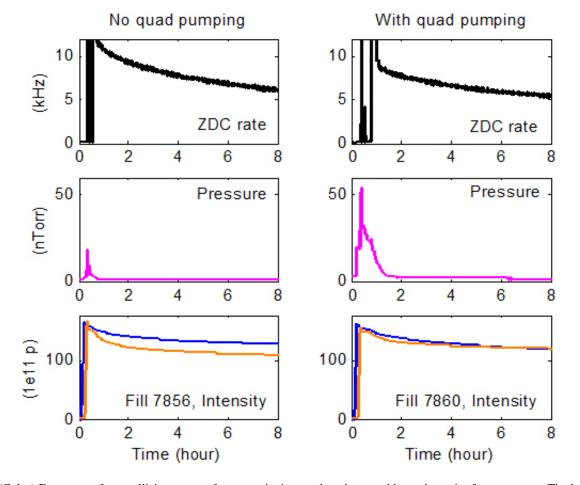
FIG. 14. (Color) Event rates from collisions, sum of pressure in 4 warm locations, and beam intensity for two stores. The left column shows the standard situation, the right column shows a store for which shorter bunches were injected from the AGS [57].
