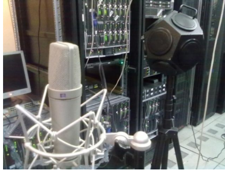
Figure 7. The power Sound source and the error microphone for data gathering to model the scndary path.
