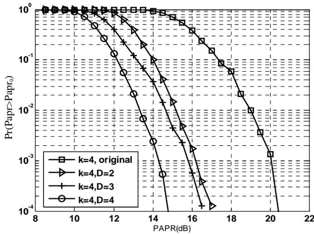
Fig. 4. *CCDF* of MC-CDMA signals using LC-VCS with  $L=64$  and different  $D$ .
