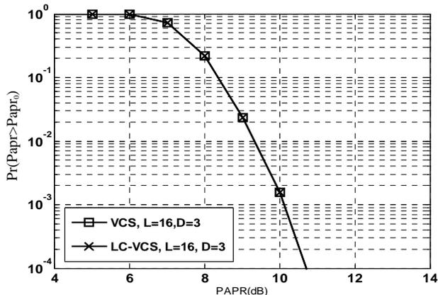
Fig. 5. Comparison of the *CCDF* of MC-CDMA signals using LC-VCS and VCS with  $L=16$ .
