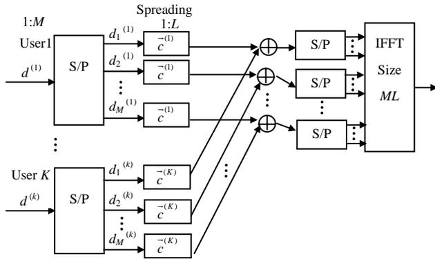
Fig.1. Conventional MC-CDMA system model
