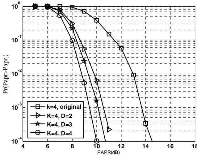
Fig. 3. *CCDF* of MC-CDMA signals using LC-VCS with  $L=16$  and different  $D$ .
