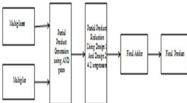
Fig. 1: Proposed Architecture of Parallel Multiplier Using Approximate Compressors.
