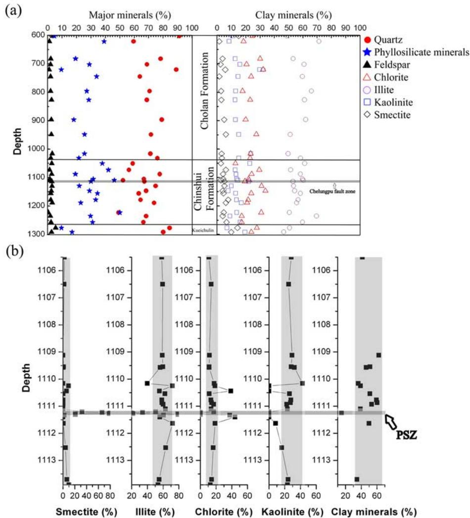
**Figure 2.** (a) Results of relative percentage of major minerals and clay minerals from TCDP cores from 600 to 1300 m in depth. (left) Plot of relative major mineral content from bulk XRD analysis. (right) Result of relative clay mineral percentage by clay mineral XRD analysis. (b) Relative clay mineral percentage and clay mineral abundance across the Chelungpu fault zone. Gray area is noted as the representative of clay content.
