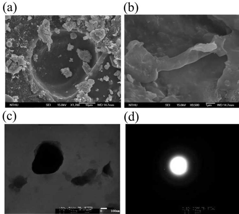
**Figure 4.** (a) SEM image of the typical surface texture of the pseudotachylyte sample in the PSZ. The image shows several vesicles or bubbles on the surface in the PSZ. (b) SEM image of pseudotachylyte displays string that is melted material drawn out when cracks opened. (c) TEM image of the grains collected from the PSZ, and (d) no light spots are evident indicating no crystal lattice in this grain. These images indeed provide evidence of melting and suggest pseudotachylyte indeed existed.
