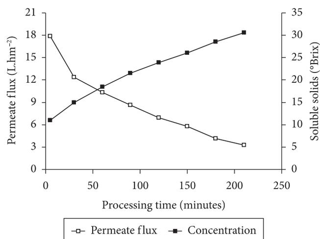
**Figure 3.** Permeate flux and concentration of soluble solids of pineapple juice in plate and frame module of reverse osmosis. Means of three assays.
