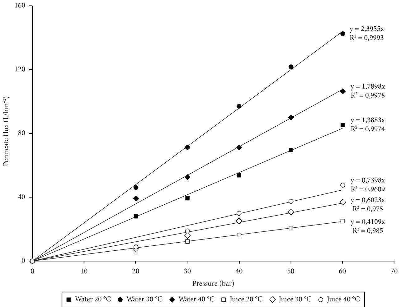
Figure 1. Permeate flux of the membrane to water and to the centrifuged pineapple juice.
