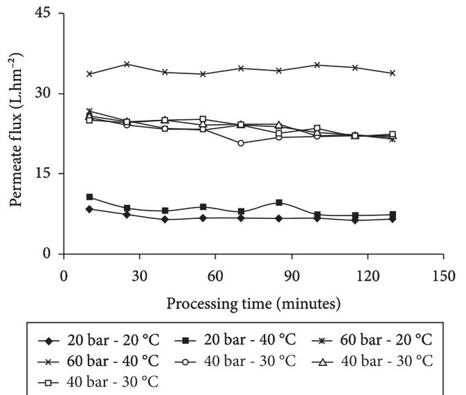
Figure 2. Permeate flux according to pressure and temperature in the stationary stage.
