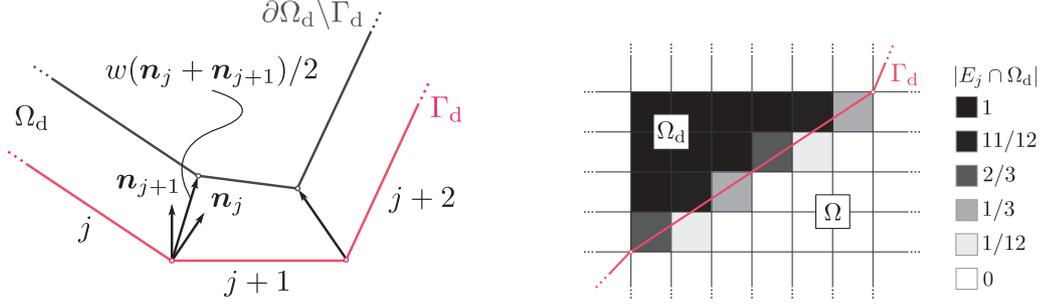
Figure 2.2: (Left) The back side of the horn is generated by linear interpolation of the points  $w(\mathbf{n}_j + \mathbf{n}_{j+1})/2$ . (Right) The values of the area  $|E_n \cap \Omega_d|$  used to find the values  $\alpha_n$  of the function  $\alpha_h$ .
