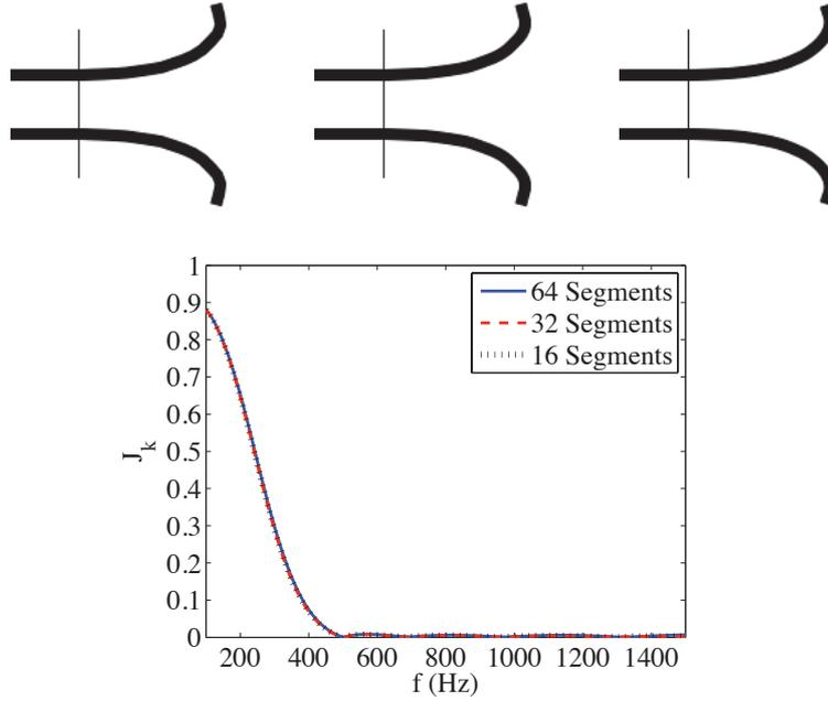
Figure 2.4: Optimal horns (top) with respect to reflections for 466–1480 Hz and their corresponding spectra (bottom). The presented pixel representations correspond (from left to right) to 16, 32, and 64 design variables and the horn length is  $|\Gamma_d| = 0.4$  m in all cases.
