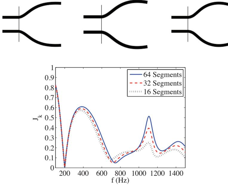
Figure 2.3: Optimal horns (top) with respect to reflections for a single frequency of 200 Hz and their corresponding spectra (bottom). The presented pixel representations correspond (from left to right) to 16, 32, and 64 design variables and the horn length is  $|\Gamma_d| = 0.4$  m in all cases.
