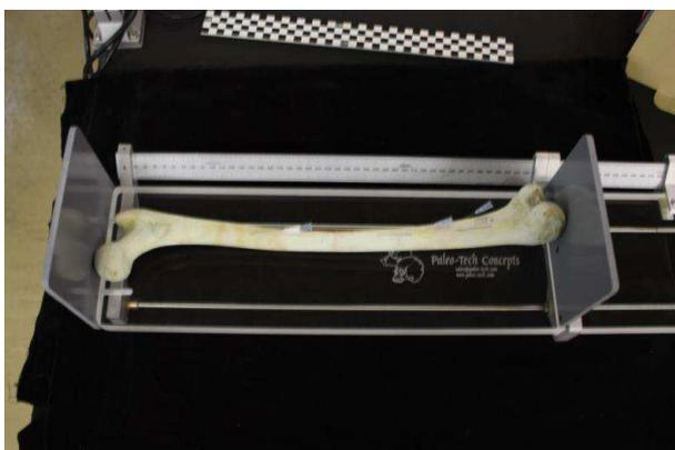
**Fig. 1.** The osteometric board used to measure the maximum length of the bones.
