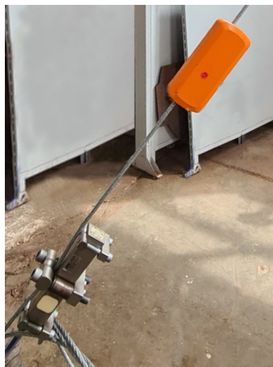
Figure 6. Photo of the leaf node and tension sensor attached to the tower cable.
