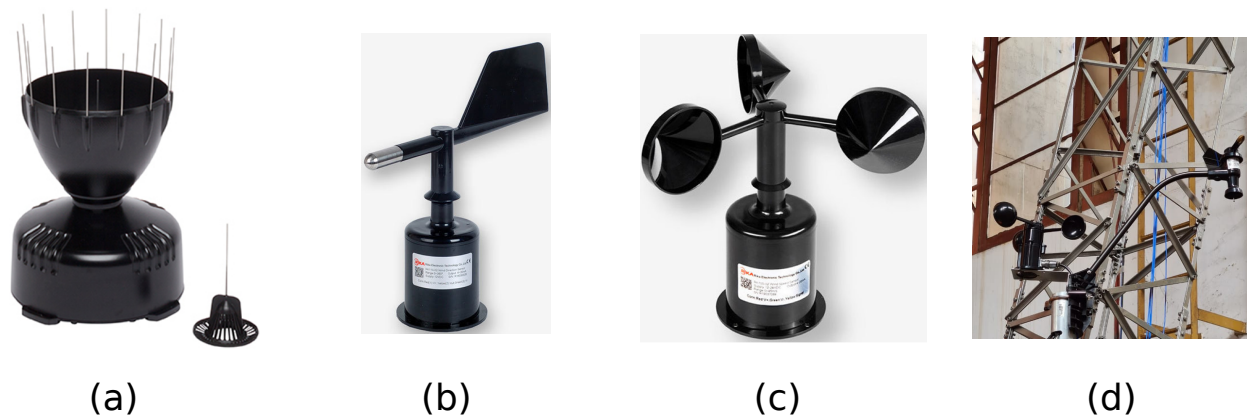
Figure 10. The weather station sensing elements: (a) rain gauge, (b) wind direction, (c) wind speed, and installed sensing elements on the mockup tower, and (d) all sensors installed in the tower.
