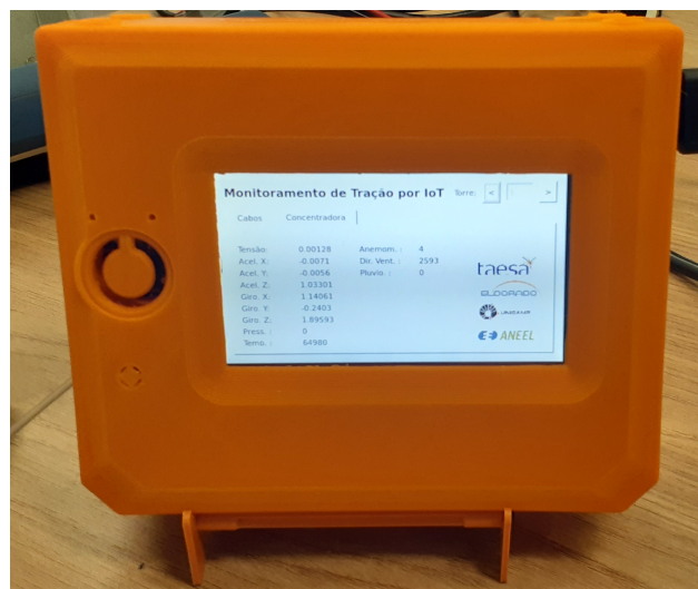
Figure 8. Photo of the border node presenting the interface of the monitored data.
