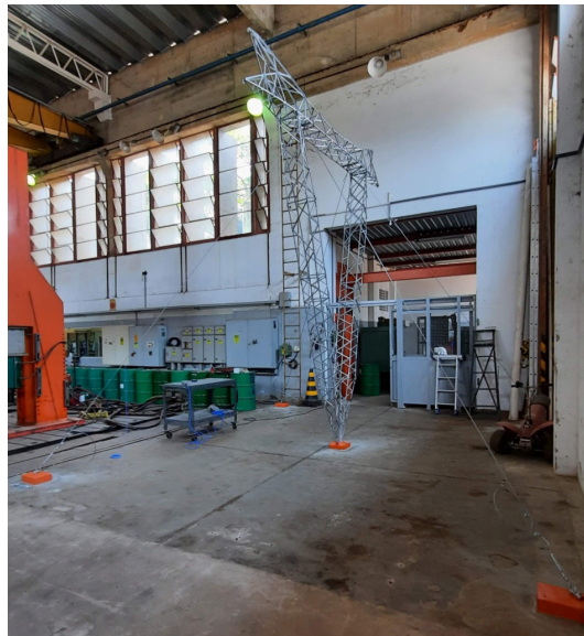
Figure 5. A photo of the mockup tower installed inside the LabEDin mechanical engineering laboratory.
