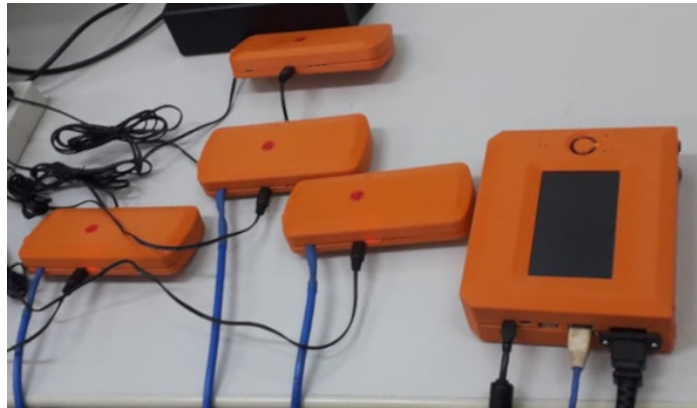
Figure 7. A photo of four router/leaf nodes and a border node being tested.
