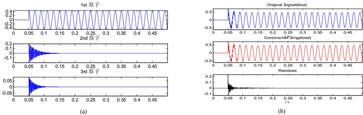
Figure 3. (a) Waveforms of decomposed atoms; (b) the reconstruction for zero sequence transient current of m line.
