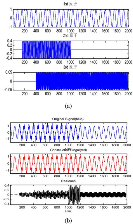
**Figure 1. (a) Waveforms of decomposed atoms; (b) the reconstruction for harmonics.**
