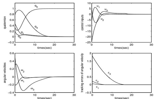
Fig.3 Simulation results in the case of  $q_0(0) \geq 0$
