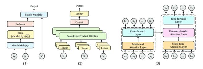
Figure 2. Transformer. (1) Scaled Dot-Product Attention, (2) Multi-Head Attention, and (3) Transformer model [24].
