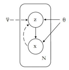
**Figure 1.** VAE. The solid line represents the generative network, and the dashed line represents the inference network [20].
