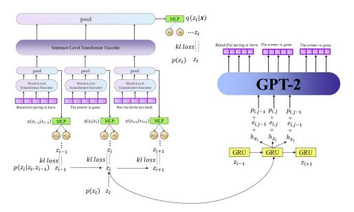
**Figure 5.** Model Architecture. The left side represents the inference network, and the right side represents the generative network.
