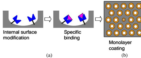
Fig. 2. Schematic of bio-molecule recognition: (a) the target molecules are captured by the probe molecules. (b) The bio-molecules form a uniform layer on the internal surface of the sensor. In reality the layer thickness is very small compared with the pore size.
