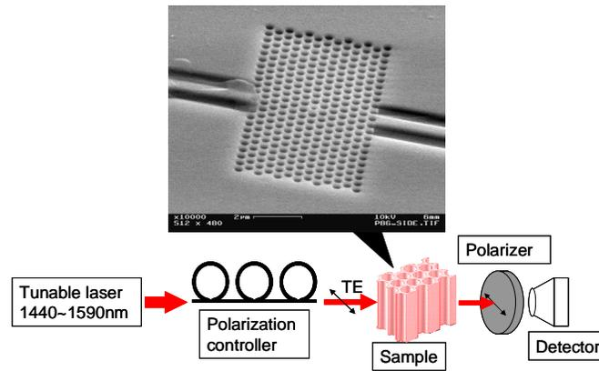
Fig. 1. Scanning electron microscopy photograph of a typical device and schematic of the experimental setup. A tunable laser (1440 nm to 1590 nm) is used as the source. Light is coupled in and out of the PC using tapered ridge waveguides. A polarization controller is used to maximize the TE mode signal, and an InGaAs detector is used to measure the transmission signal.
