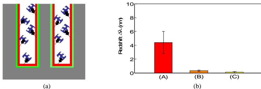
Fig. 6. (a) Schematic of biotin-streptavidin binding recognition. (b) Amount of resonance redshift resulting from device exposure to different solutions. Bar (A) shows the amount of redshift resulting from specific binding of streptavidin to biotin. Bar (B) shows that the contribution to the shift from non-specific binding (no probe molecule) is negligible. Bar (C) shows that there is no contribution by the buffer alone.
