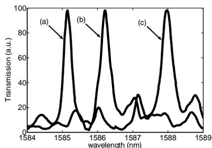
Fig. 3. Normalized transmission spectra of the PC microcavity. Curve (a) indicates the initial spectrum resonance after oxidation and silanization, curve (b) is measured after glutaraldehyde attaches to the pore walls, and curve (c) is obtained after infiltration of BSA molecules.
