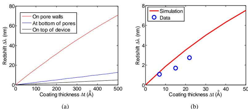
Fig. 4. (a) Calculated resonance redshift versus the monolayer coating thickness on the pore wall, bottom, and top of the device. (b) Red curve shows the calculated resonance redshift versus the coating thickness on the pore wall. Blue dots show the protein layer thicknesses measured by ellipsometry. The ellipsometric data are in agreement with the model.
