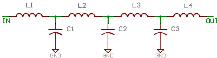
Fig 2. The 7 poles circuit design by filter calculator
