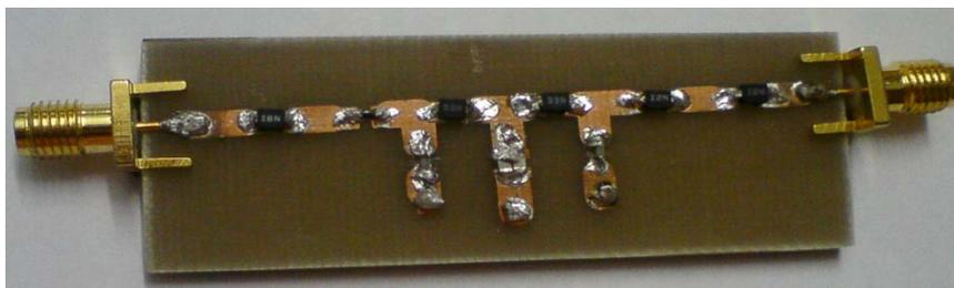
Fig 10. Hardware Butterworth low pass filter
