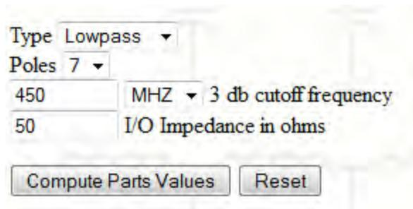
Fig 1. Instruction of Design an L-C low pass or high pass filter
