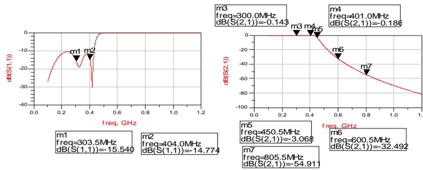
Fig 6. Simulation S-parameter result after tuning
