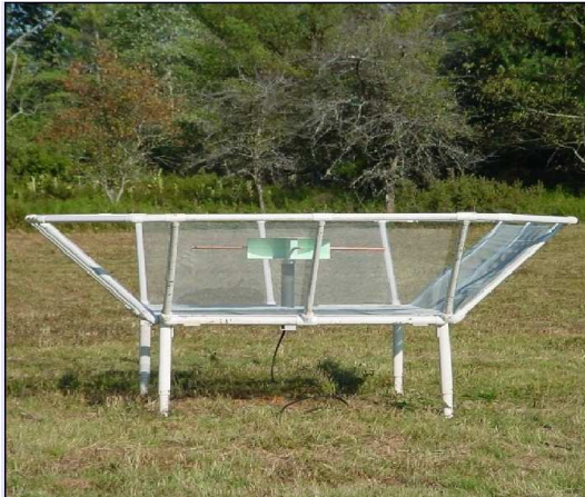
FIG. 7: PAPER antenna. The ground screen structure includes side reflectors that narrow the size of the primary beam to more closely match the size of colder patches in the synchrotron sky.
