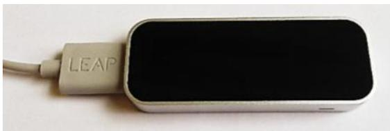
Fig.1 Leap Motion Sensor
