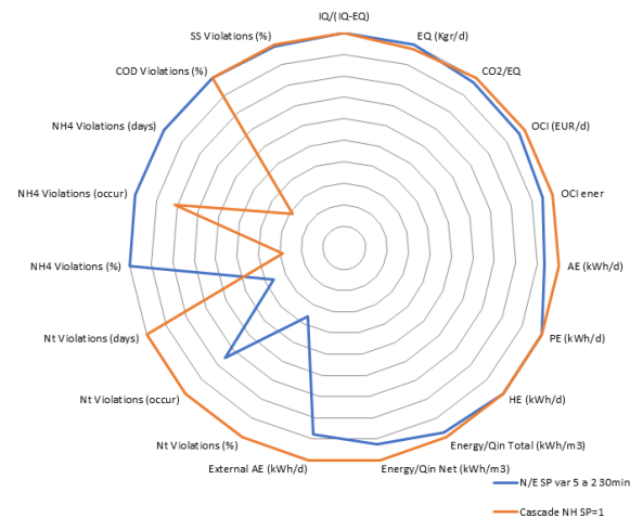
Figure 17. Radar plot of performance indicators for the comparison between Cascade SP_{NH} = 1 and N/E control strategy.
