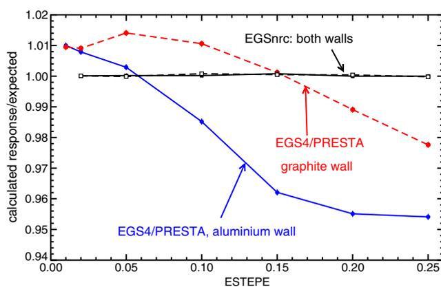
**Figure 4.** Verification that EGSnrc accurately calculates the response of graphite and aluminium-walled pancake ion chambers irradiated by a  $^{60}\text{Co}$  beam at the 0.1% level whereas EGS4/PRESTA failed by 1%, even for very small step sizes. ESTEPE is the maximal fractional energy loss allowed per electron step. From front cover of the EGSnrc manual (Kawrakow and Rogers 2000) based on data from (Kawrakow 2000b).
