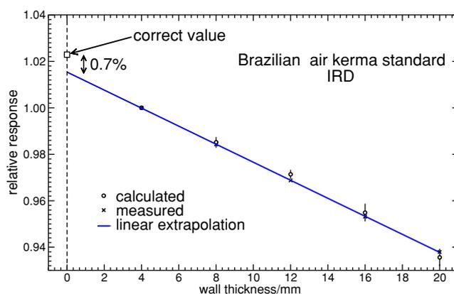
**Figure 3.** Comparison of calculated and measured responses of the Brazilian primary standard for air kerma as a function of the wall thickness and the linear extrapolation to zero wall thickness used to determine  $A_{\text{wall}}$  compared to the value obtained from direct Monte Carlo calculations of  $A_{\text{wall}}$ . Redrawn from data in Rogers and Bielajew (1990b).
