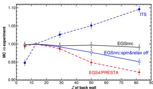
**Figure 5.** EGSnrc simulations of a parallel-plate ion chamber's response in a broad parallel  $^{60}\text{Co}$  beam as a function of the atomic number of the replaceable back wall. Results are divided by the experimental data of Nilsson *et al* (1988) (which has an uncertainty of 0.5%) and normalized to unity at  $Z = 13$ . From Kawrakow and Rogers (2001).
