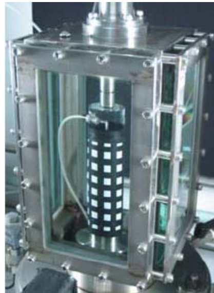
Fig 1. Sketch map of laboratory test of conditioned soil for tree-dimensional compression
