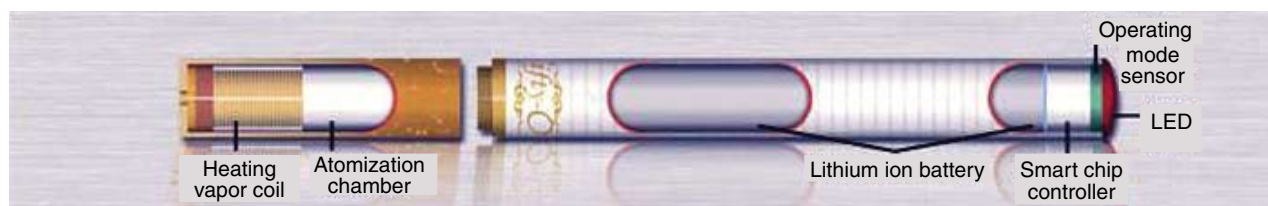
Figure 1. Basic design of an electronic cigarette.
