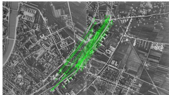
Figure 7: The result after executing the PUMA algorithm. Out of 218 putative matches 34 were chosen as inliers.
