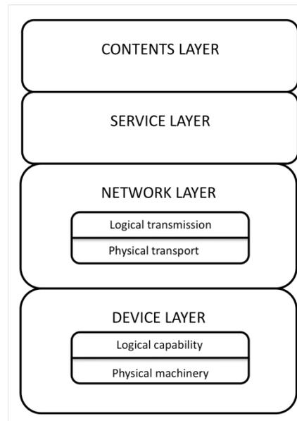
**Figure 1. The Layered Architecture of Digital Technology**
