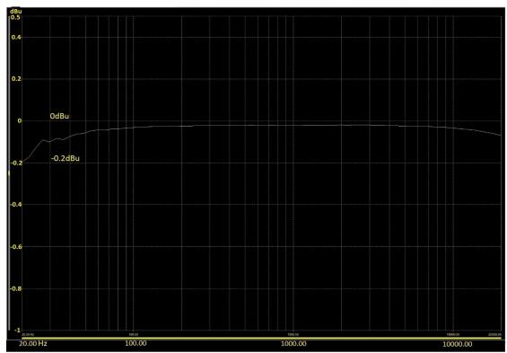
Figure 9: Solid-State Frequency response
