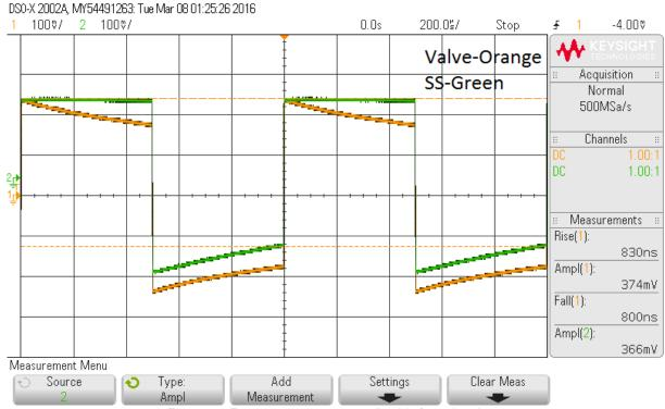
Figure 13: Frequency response predictable from the slopes
