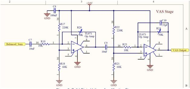
Figure 3: Solid-State Voltage Amplification Stage
