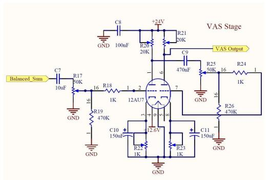
Figure 4: Valve Voltage Amplification Stage
