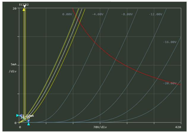
Figure 5: Valve Load-Line
