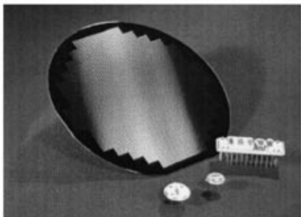
Fig. 8 Acoustic wave sensors are commercially available in several form factors. Most sensors begin as processed wafers, and then are tested, diced, and mounted into packages (Photo Courtesy Microsensor Systems Inc.).
