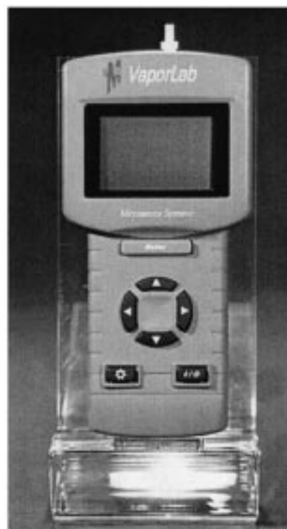
Fig. 13. Commercially available SAW chemical vapor analyzer. This handheld analyzer utilizes an array of four SAW sensors, each coated with a different polymer (Photo Courtesy Microsensor Systems Inc.).
