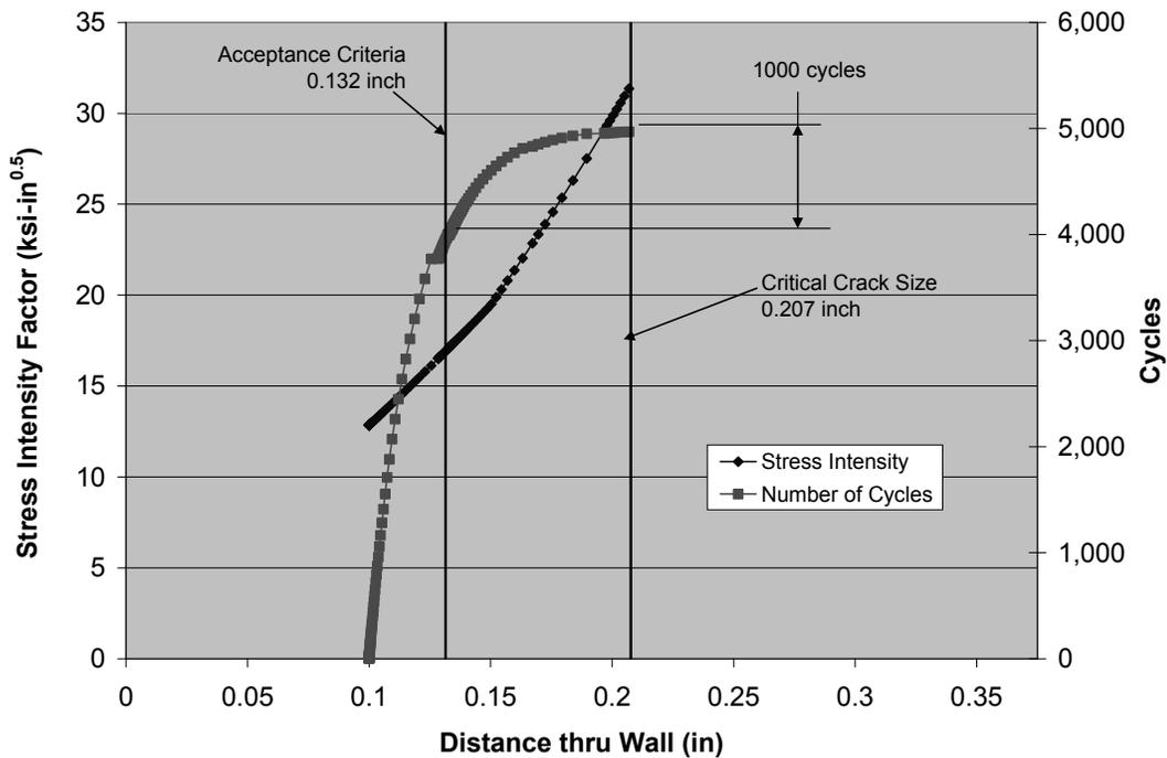
FIGURE 2 – CRACK GROWTH STUDY OF SUPPLY TUBE BEND
