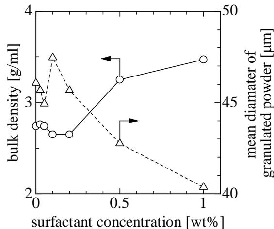
Fig.6 Dependency of surfactant concentration on properties of granulated powder
