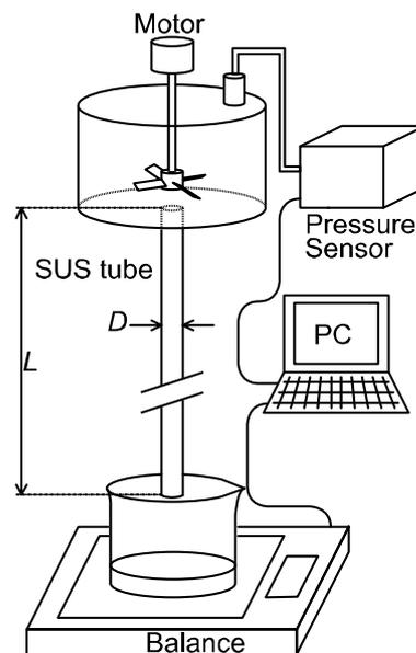
Fig.1 Schematic of vertical capillary tube viscometer
