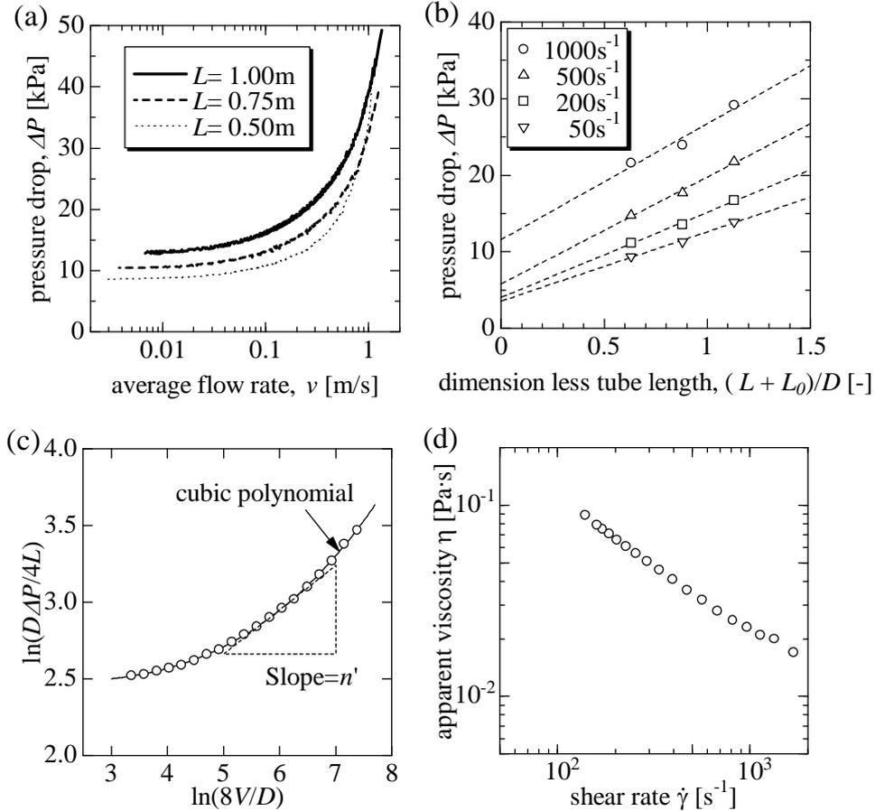
Fig.2 procedure for pressure drop calculation
