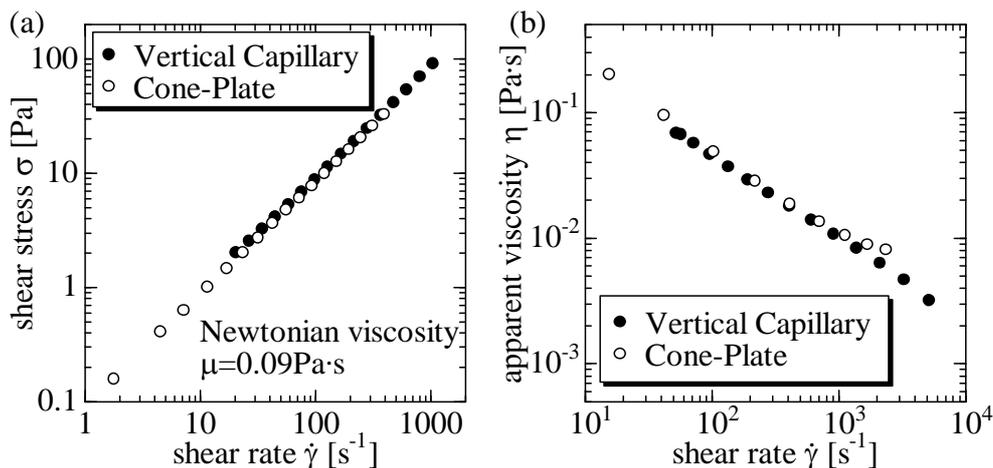
Fig.3 Rheological comparisons between results of vertical capillary tube and cone plate rheometer
