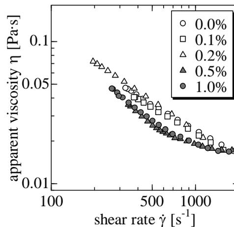
Fig.4 Dependency of surfactant concentration on rheological characteristics of suspension
