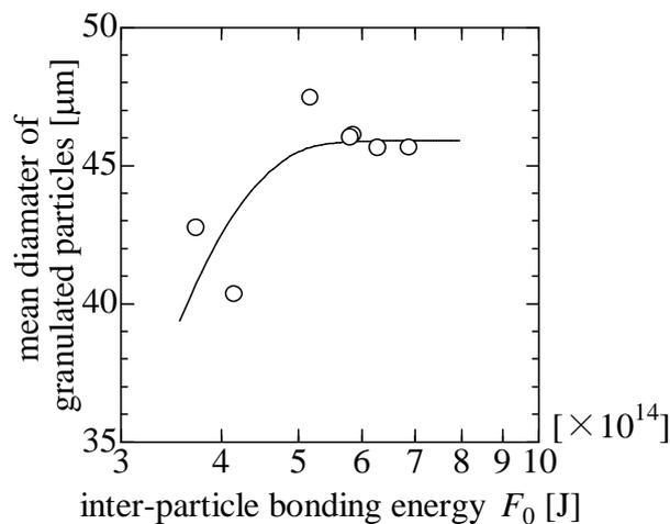
Fig.7 Relationship between granulated particle size and particle interaction
