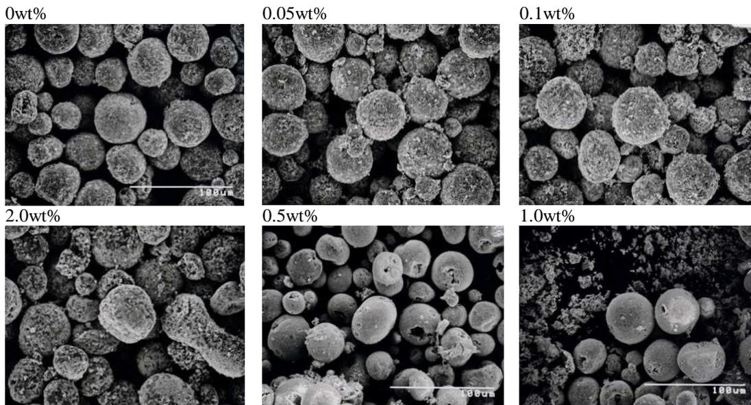
Fig.5 External appearance of granulated powders with different surfactant concentrations
