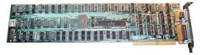
Fig. 3: IBM PC's monochrome display adapter
