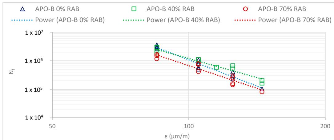
Figure 5. Fatigue curves ( $N_{f50}$ ) of the three asphalt mixtures.
