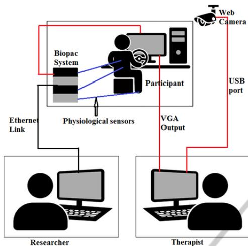
Figure 3: Experimental setup diagram.
