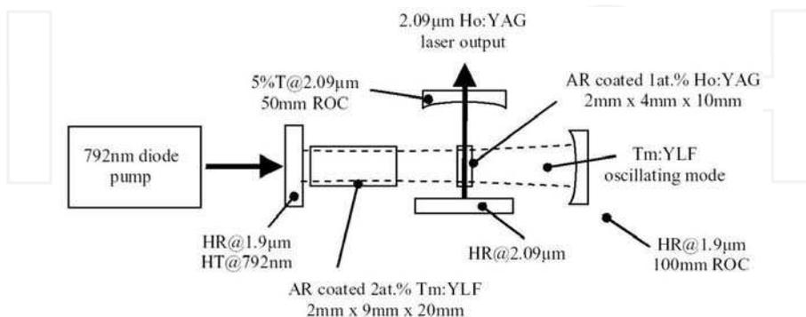
Fig. 7. Schematic diagram of a Ho:YAG intra-cavity pumped laser (So et al., 2006)
