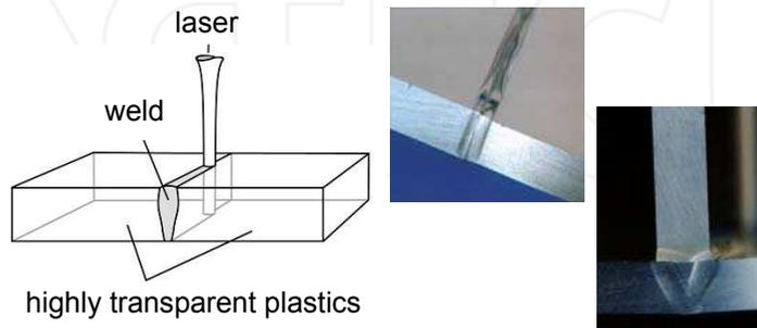
Fig. 19. Left side: Schematic diagram for welding two highly transparent plastics with a butt joint. Right side: Welding examples prepared with a 2  $\mu\text{m}$  Tm:YAG laser by Prolas GmbH, Aachen (butt joint 4 mm PMMA and T-bonding 3 mm PMMA)
