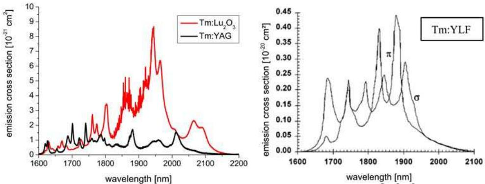
Fig. 4. Left side: Emission cross sections of Tm:YAG and Tm:Lu<sub>2</sub>O<sub>3</sub> for the transitions from the  ${}^3\text{F}_4$  manifold to the ground state (Koopmann et al., 2009b). Right side: Emission cross sections for  $\pi$  and  $\sigma$  polarisation of Tm:YLF (Budni et al., 2000).
