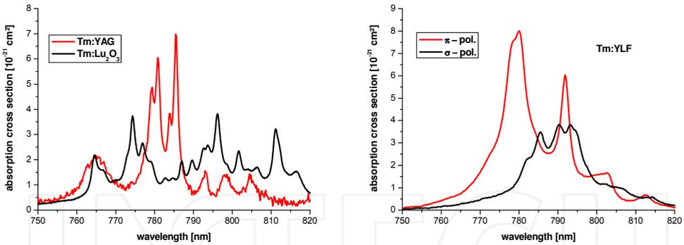
Fig. 3. Absorption cross sections of the  ${}^3\text{H}_6 \rightarrow {}^3\text{H}_4$  transition for Tm:YAG, Tm:Lu<sub>2</sub>O<sub>3</sub>, (Koopmann et al. 2009b) and Tm:YLF.
