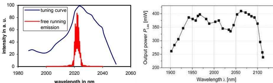
Fig. 5. Tuning curves of Tm:LuAG (Scholle et al., 2004) and Tm:Lu<sub>2</sub>O<sub>3</sub> (Koopmann et al., 2009a)
