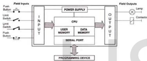
**Fig 2.1 Architecture of PLC**
