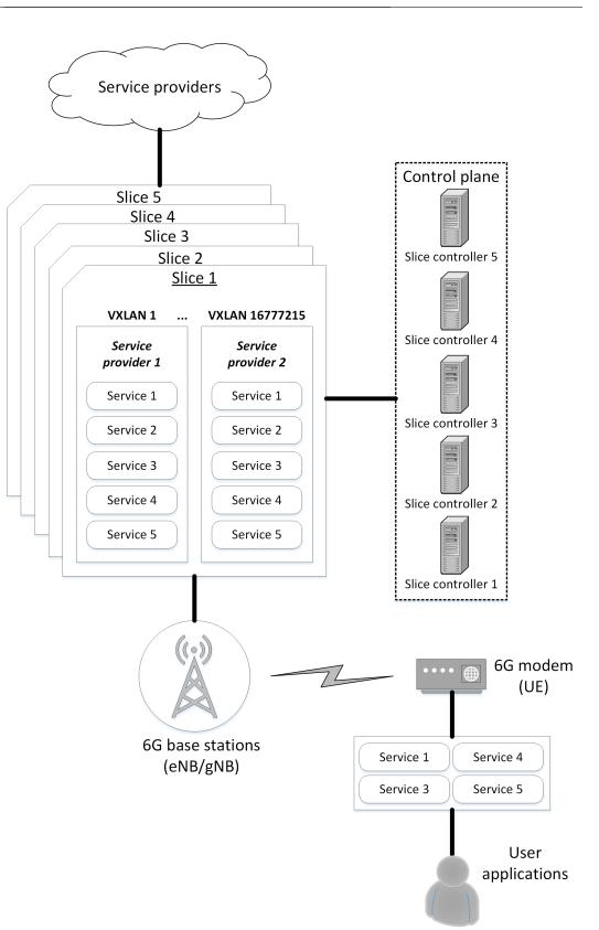
Figure 2. Service bonding and provider isolation in a multi-slice environment.
