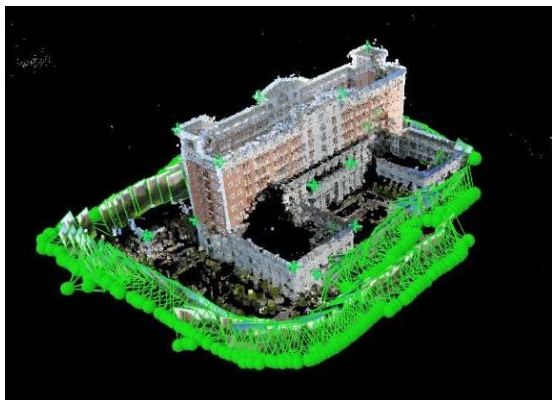
Figure 7. Point cloud of the building generated by Pix4Dmapper.
