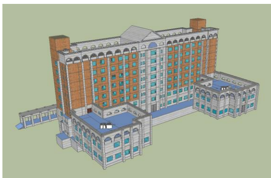
Figure 8. Building model generated from the point cloud by AutoCAD 2016 and SketchUp Make 2016.
