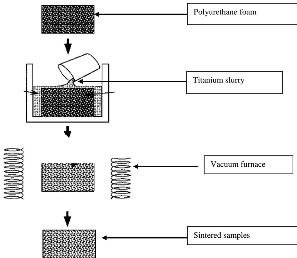
Figure 3 Schematic Illustration of the Production of the Titanium Foam
