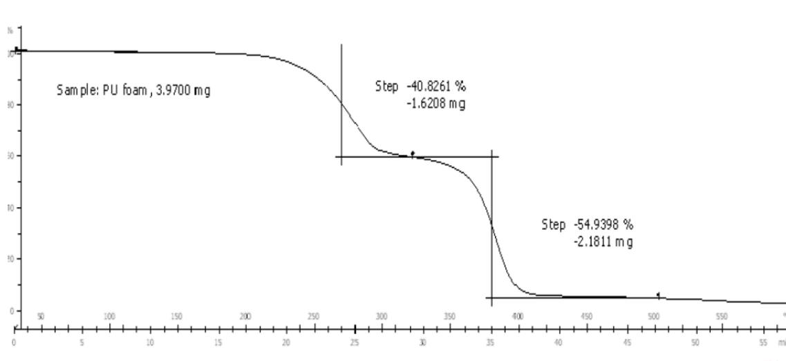
Figure 4 TGA Analysis of the polyurethane Foam
