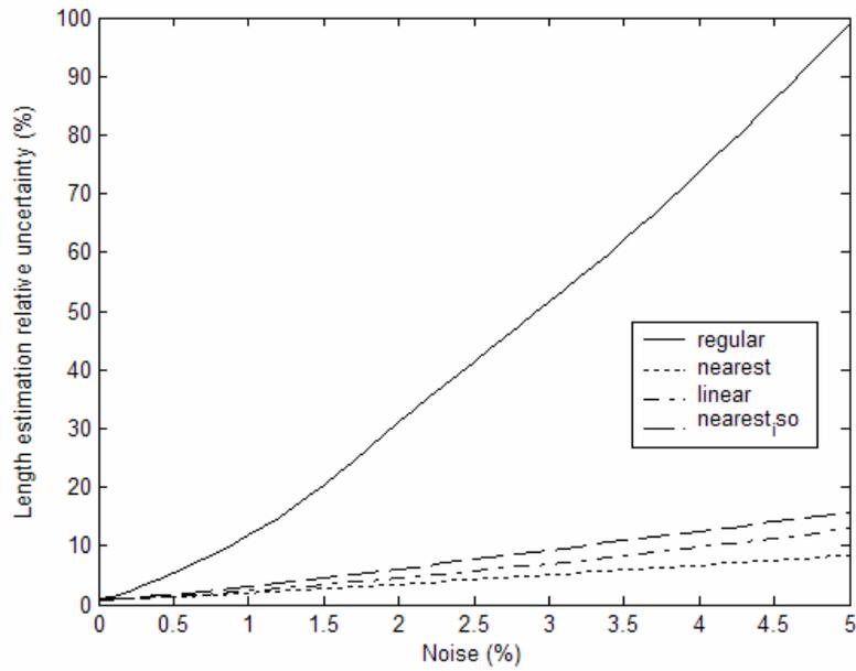
**Fig. 7.** Length estimation uncertainty of neural networks trained with different training sets for ID cracks
