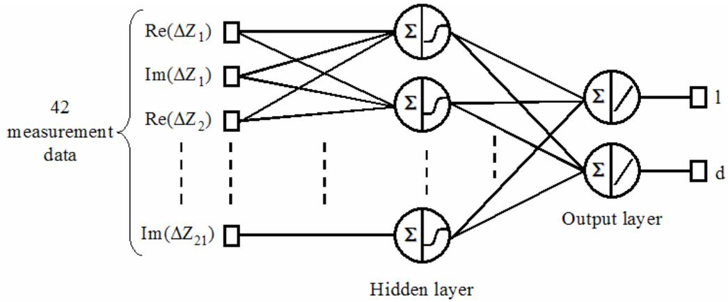
**Fig. 4.** General structure of the implemented neural networks
