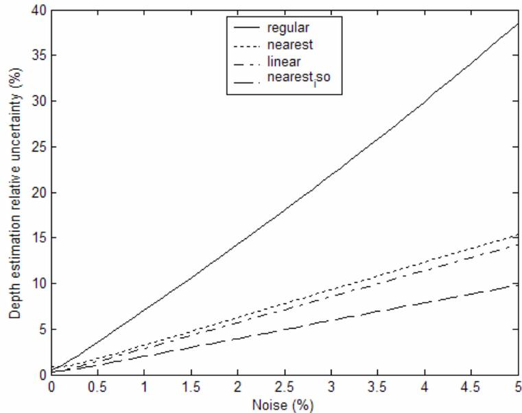
**Fig. 8.** Depth estimation uncertainty of neural networks trained with different training sets for ID cracks
