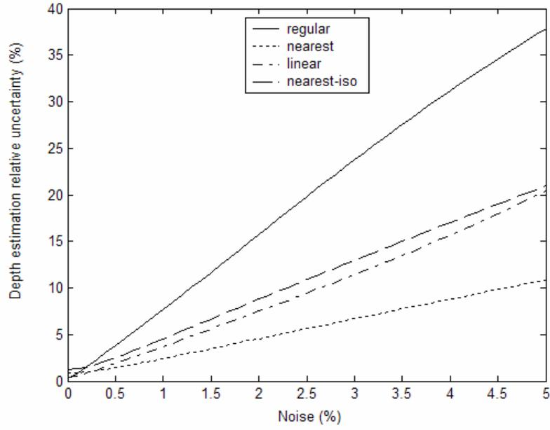
**Fig. 6.** Depth estimation uncertainty of neural networks trained with different training sets for OD cracks
