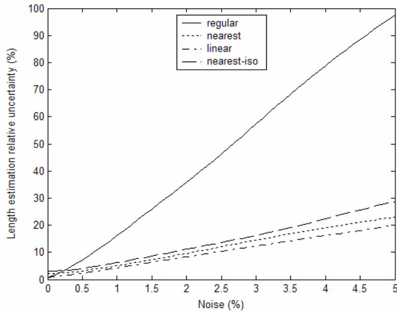
**Fig. 5.** Length estimation uncertainty of neural networks trained with different training sets for OD cracks
