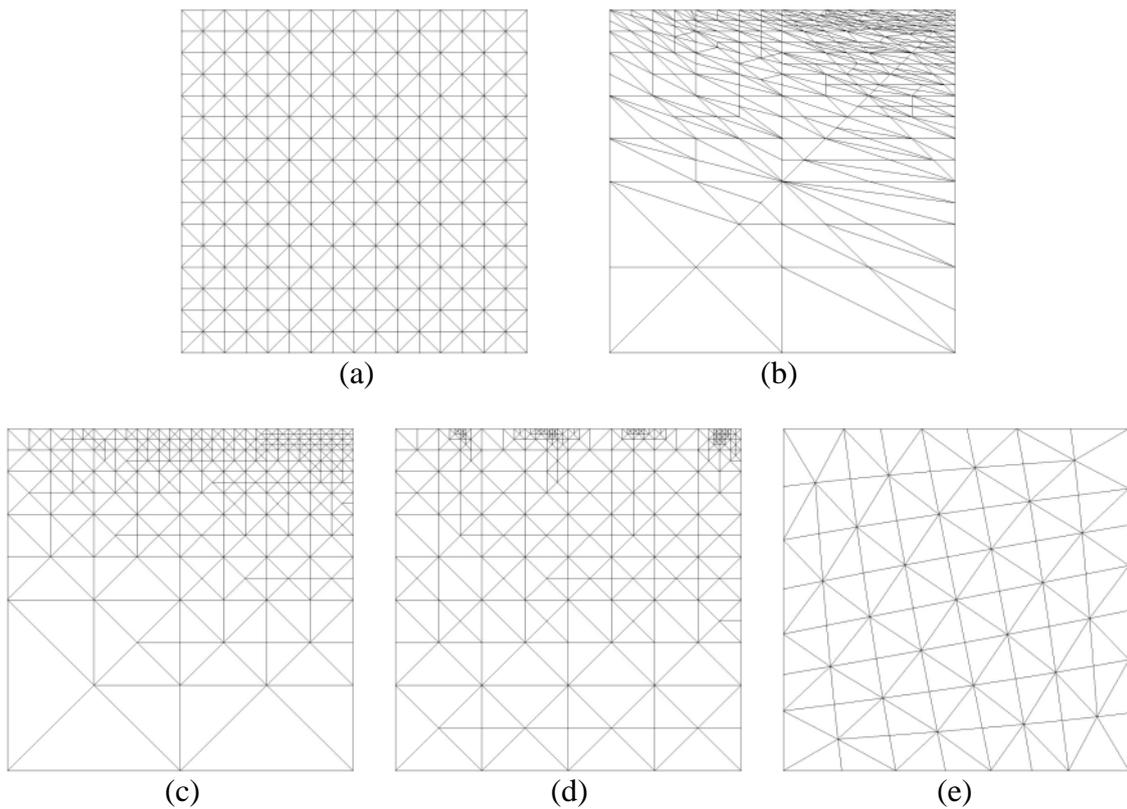
**Fig. 2.** Distribution of the database examples in the parameter space for OD type cracks: uniform sampling (a); optimised for nearest neighbour interpolation (b); the same with triangle shapes constrained (c); optimised for linear interpolation (d). Test data set (e).
