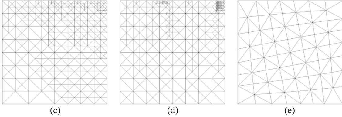
**Fig. 3.** Distribution of the database examples in the parameter space for ID type cracks: uniform sampling (a); optimised for nearest neighbour interpolation (b); the same with triangle shapes constrained (c); optimised for linear interpolation (d). Test data set (e).
