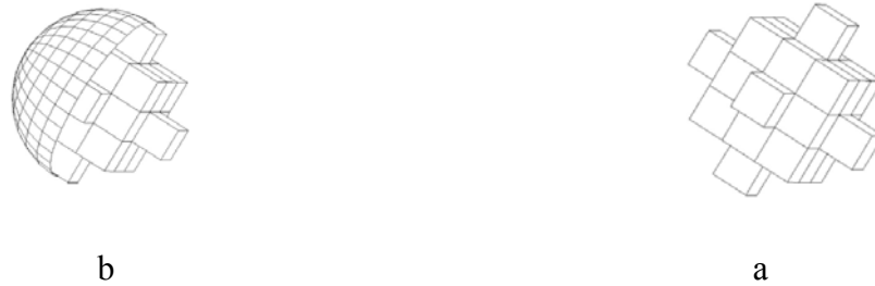
Fig. 6. The transmission space of a sensor node, (a) Logically transmission range. (b) Physically transmission range.
