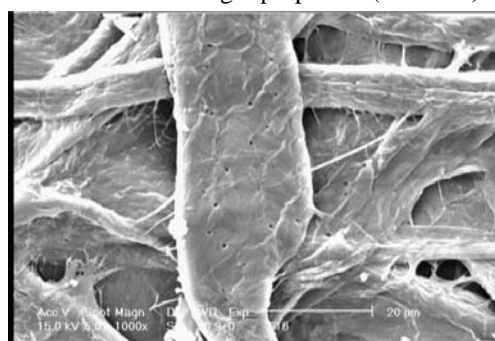
Fig. 1 SEM micrograph refined recycled fibers with magnification 1000x
