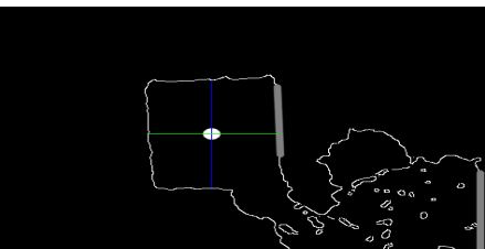
Figure 4: From the tracked (x,y) position, find edges above, below, and to the sides. The new (x,y) tracked point is the centroid of these four points. For objects with smooth borders, this operation converges to a point over time.
