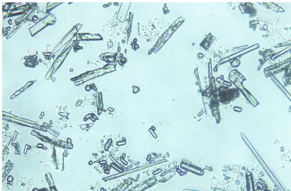
Figure 12: Hexagonal crystals from bottom layer of crucible
