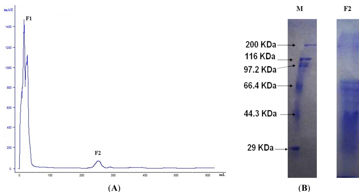
**Figure 2.** Affinity chromatography using Celangulin V-Sepharose of BBMV proteins extracts from *M. separata* larvae. (A) F1 is the unbound protein eluted with binding buffer; F2 is eluted with Celangulin V dissolved in binding buffer; (B) 12% SDS-PAGE of fraction M: protein marker; F2: Fraction 2.
