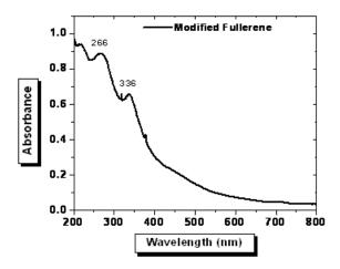
Figure 4.Optical absorption of pure Modified Fullerene film spin-coated from chloroform.
