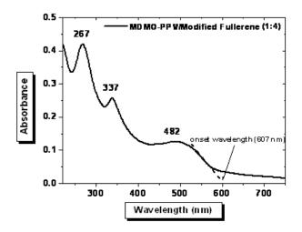
Figure 5. Optical absorption of MDMO-PPV: Modified Fullerene (1:4) film spin-coated from 1, 2diclorobenzene.
