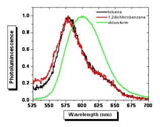
Figure 3. The PL spectra of pure MDMO-PPV film spin-coated from toluene, 1,2dichlorobenzene and chloroform.
