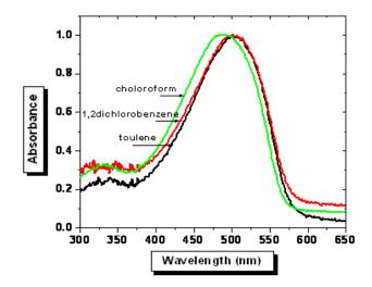
Figure 2. The UV-vis spectra of pure MDMO-PPV film spin-coated from toluene, 1,2dichlorobenzene and chloroform.
