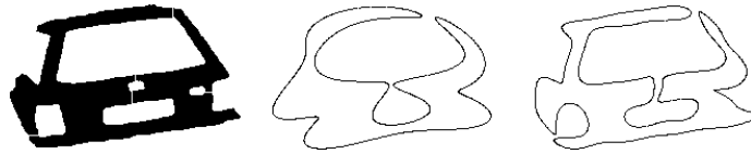
Figure 7. (a) Cut region silhouette, Boundary reconstruction from (b) 10 coefficients, (c) 30 coefficients
