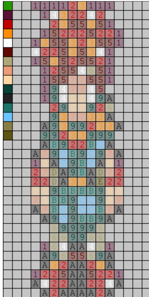
Figure 4.3c: Zoom in on Figure 4.3a, with pixel values. Zero omitted for clarity. Palette on the left-hand side.
