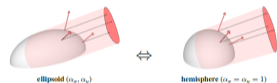
Figure 1. Sampling the GGX distribution of visible normals (VNDF) is equivalent to sampling the projected area of an ellipsoid, which can be mapped to sampling the projected area of a hemisphere.
